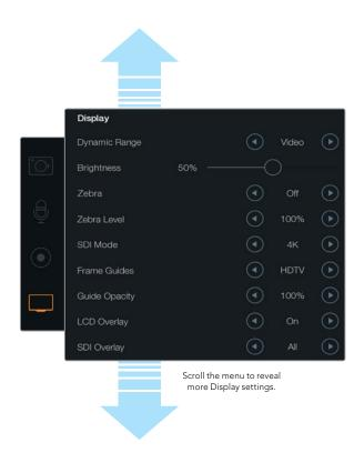
The 'display' settings screen on Blackmagic Production Camera 4K. Display settings on Blackmagic cameras lets you set the brightness of the LCD, turn LCD overlays on or off, adjust the display dynamic range and zebra settings. You can also choose what overlays are visible on your camera's SDI or HDMI output and select your desired frame guides.
