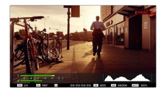
In Blackmagic Micro Cinema Camera, the status strip and on screen meters can be viewed on the HDMI or composite output display.
