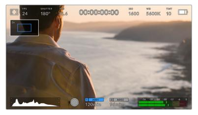
While zoomed in, an indicator in the top left of your LCD touchscreen will show which part of the image you are viewing. You can move around the image by dragging your finger along the screen as you would on a smartphone or tablet
