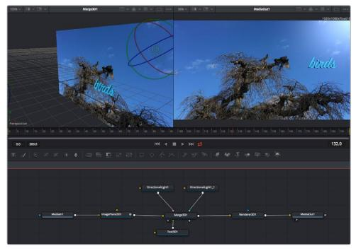
The most commonly used tool is the 2D or 3D merge node. This node is like a central hub that combines tools on the node editor into a single output.
