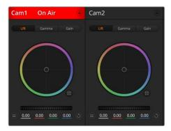
Each camera controller displays the channel status so you know which camera is on air. Use the color wheels to adjust each YRGB channel's lift, gamma and gain settings
