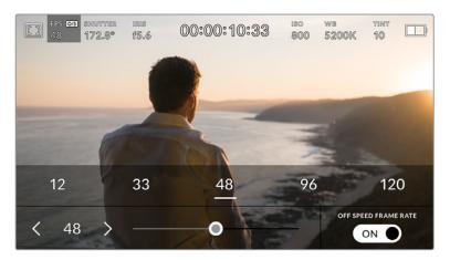
With 'off speed frame rate' enabled, tap the arrows on either side of the sensor frame rate, move the slider or tap one of the presets to make adjustments
