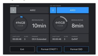
When an SSD is inserted into URSA Mini SSD Recorder, your camera's storage manager will display 'SSD Recorder' over storage slot 2.
