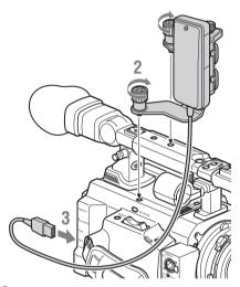
**3** Connect the USB cable of the CBK-WA01 to the Option connector (USB A connector) on the PMW-F3K/F3L.
