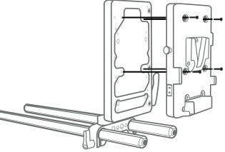
NOTE: To change BATTERY SLIDE position loosen THUMB SCREW and slide into desired position
