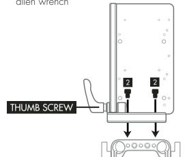
For attaching to battery mount find appropriate threaded holes by using the HOLE CHART below. Insert and tighten PHILLIPS HEAD SCREWS into corresponding hole as shown on HOLE DIAGRAM.
