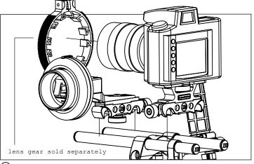
Attach Lens Gear / Follow Focus / Camera Assembly 4a: Attach Lens Gear to Camera Lens 4b: Attach Follow Focus to CF Rods 4c: Attach Camera / DSLR Baseplate Assembly to CF Rods HELPFUL HINT: Lens Gear and Follow Focus need to be aligned properly. Make sure that Gear / Follow Focus / Camera
