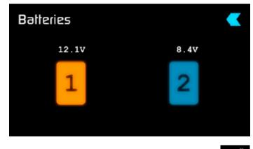
In the picture above we see Battery 1 is full and active and Battery 2 is currently inactive and 1/4 depleted. If no battery is present it will show an X in the picture and will be Black in colour as pictured right.
