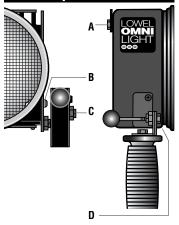
Omni has four constant-tension (torque) pivot points. All have flat spring washers to maintain proper tension and can be adjusted, if necessary, with a 7/16" wrench.
