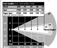
Beam angles-points at which intensity drops to
