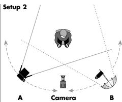
**Setup #2** uses 2 Omni's, one with only barn doors, as hard key, and the other with a Tota-brella as soft fill. Vary the position of the lights, as shown. Be aware of reflection in eyeglasses or reflective surfaces.
