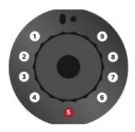
The function of each switch is divided into short presses (less than  $\frac{1}{2}$  second), and long presses (hold more than  $\frac{1}{2}$  second).
