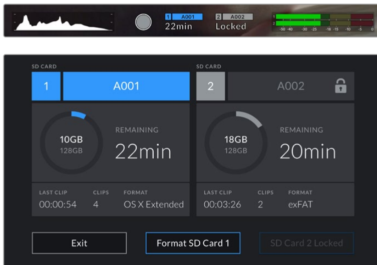
Your URSA Broadcast will indicate when locked SD storage media is inserted
