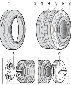
**Note:** The rear cap included with the lens that comes with the lens kit may differ from that shown, in which case it can be removed without performing Step ①.
