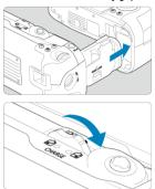
Insert the battery in the camera and turn the release dial to lock the battery grip in place.
