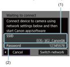
Check the SSID (1) and password (2) displayed on the camera screen.
