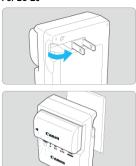
As shown by the arrow, flip out the battery charger's prongs and insert the prongs into a power outlet.
