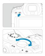
Press a button such as < MENU >, then turn the < \$\sum\_{y=0}^{\infty} > \text{dial.} If you press the shutter button halfway, the camera will go back to
