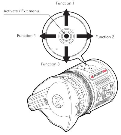
Press the joystick to activate the menu. Press the joystick again to exit the menu.
