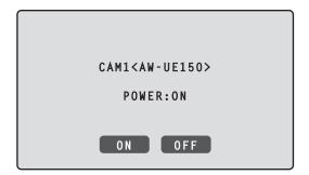
Turning on the power of the cameras simultaneously with the turning on of the unit's power
