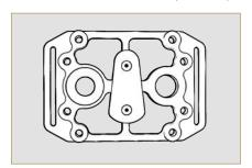
Slide the plate into the Pop-n-Lock base to mount the transmitter to the MōVI Pro. 3.
