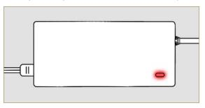
5. When the AC power adapter's LED returns to GREEN, your battery is fully charged. Press the power button on the battery to check the power level, and disconnect the battery from the charger.
