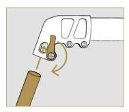
2. Place MōVI Pro on a MōVI Dock and use four M3 screws to attach the front landing gear to the front of the MōVI Pro's Pan arm.
