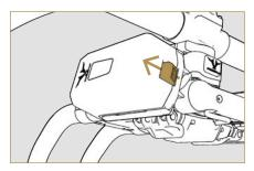
4. To hot swap MōVI Pro batteries, simply remove and replace the batteries one at a time.
