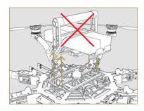
**3.** Attach the MōVI Pro to the top of the ALTA and lock into place using the upper TITH connector.
