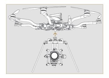
2. Lock the TITH to secure the MōVI Pro in place, and the MōVI is now flight ready!
