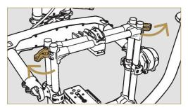
2. Open the top and bottom camera rail toggle clamps, and rotate the top toggle 90 degrees counterclockwise.
