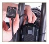
3. Ensure the 5 pin connector from the MIMIC Beta is plugged into the MIMIC TX. Power the MIMIC Beta by connecting the USB to the battery and the 3-pin connector to the MIMIC Beta.
