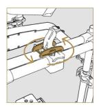
**3.** Position the camera package so the camera rail and dovetail are aligned, and then slide the camera package onto the dovetail.
