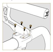
**6.** Attach your MōVI Pro using the TITH and confirm that the TITH is properly engaged and secured.
