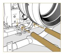
**4.** Mount and position your FIZ motors on the carbon rods so the gears interlock fully with their respective lens gears. Tighten the FIZ motor onto the carbon rod.
