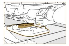
Rotate the latch on the Pop-n-Lock to secure the transmitter. 4.
