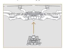
**2.** Remove the Quick Release Top Handle by disconnecting it from the TITH connector on top of the ALTA.
