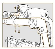
3. Slide the rear landing gear into the slot underneath the GCU from either side and secure it with two M3x8 screws.
