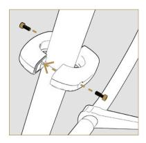
**5.** Use the (4) M3x6 screws to attach the MōVI Pro Low Profile Handle to the Ring Pro to it faces in the same direction as the MōVI Ring Pro feet.
