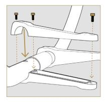
**a.** Make sure that the foot is orientated outward and has a forward lean of 4° from horizontal.
