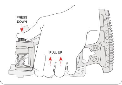
WITH THE GUNSTOCK ARM LIFTED, ROTATE THE ARM 180° INTO THE OPEN POSITION AS SHOWN.
