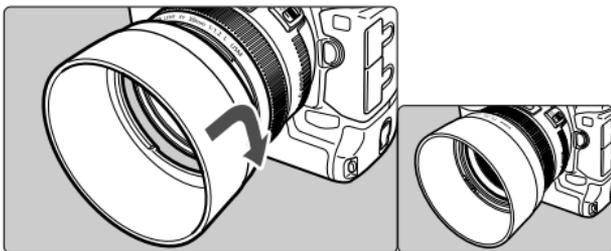
The ES-78 hood can keep unwanted light out of the lens, and also protects the lens from rain, snow, and dust.
