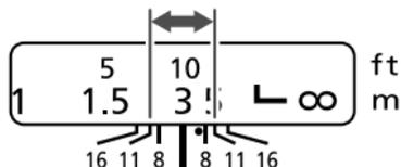
The depth of field is the distance in front of and behind the plane of focus on the subject that appears sharp. The depth of field is indicated by the area between the depth-of-field scale lines below the distance scale. Numbers in the scale are in F values, and for example, if the shooting distance is 3m and the aperture is f/11, the sharp area will extend from about 2m to 5m.
