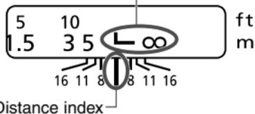
To compensate for shifting of the infinity focus point that results from changes in temperature. The infinity position at normal temperature is the point at which the vertical line of the L mark is aligned with the distance indicator on the distance scale.
