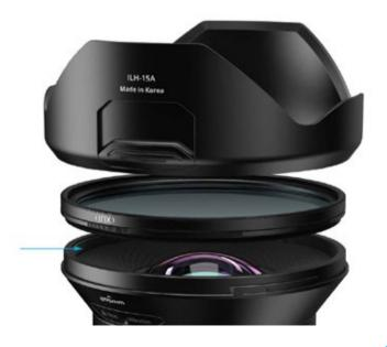
Your Irix lens can accept 95 mm screw-in filters via the front threads. Due to the wide angle of view, the use of "slim" filters is advisable to prevent vignetting. Filters with a low profile of 5.3 mm or less are recommended. Stacking multiple filters may also cause vignetting.
