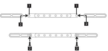
3. Select the two HANDLES, locate and align the 1/4-20 HOLES to SIDE BRACKETS as shown below, select and tighten 1/4-20x1/2" SCREWS with allen wrench
