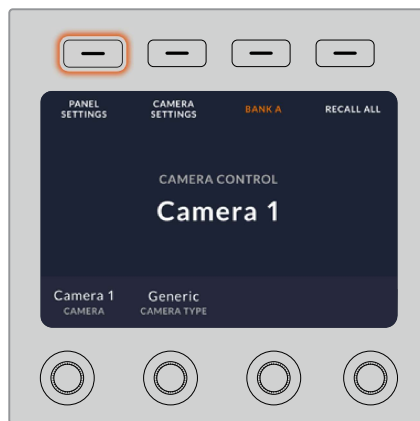
Press the 'panel settings' soft button on the LCD home screen to access all the camera control panel's settings
