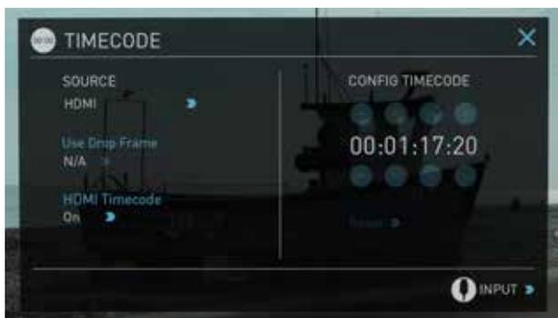
With this setting, the HDMI input will use the Timecode embedded in the input signal. The controls to adjust the Timecode value are disabled in this menu as you will need to adjust these on the camera. Note that not all HDMI sources embed Timecode.
