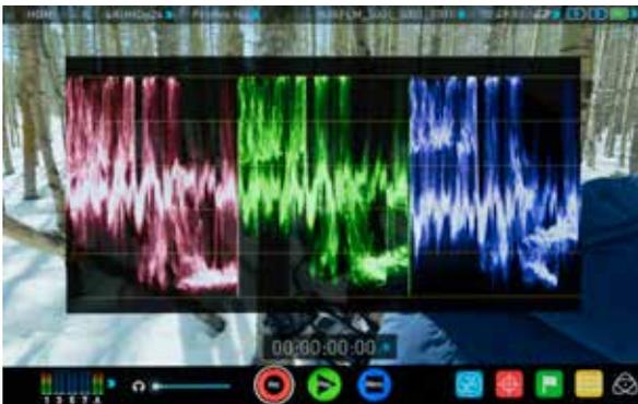
RGB Waveform will monitor the level of Red, Green and Blue from an input source. The RGB channels are displayed side by side. This can be used to check to white balance. Just point the camera at something white and the Red, Green and Blue levels should match if white balance is setup correctly on the camera.
