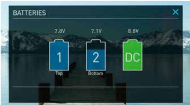
The Batteries screen indicator is made up of three icons, two will display the batteries and the other for the DC input. The active battery is shown in green and the level of the battery is shaded in 1/4 increments with a voltage level shown on top.
