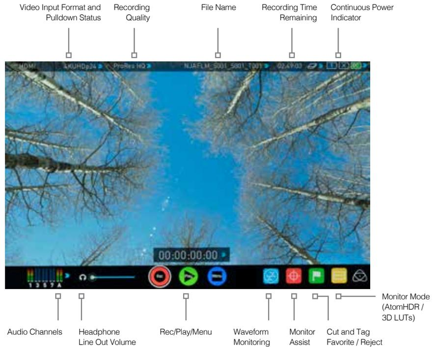
**🚩** Touching the center of the screen at any time removes the top interface overlay, tapping again clears the bottom controls and a third tap brings all the options back up. Active Shot Setup or Monitor assist functions that are enabled will remain active when the menu system is cleared. This is to allow you to use the Shot Setup and Monitor assist functions at all times while shooting.
