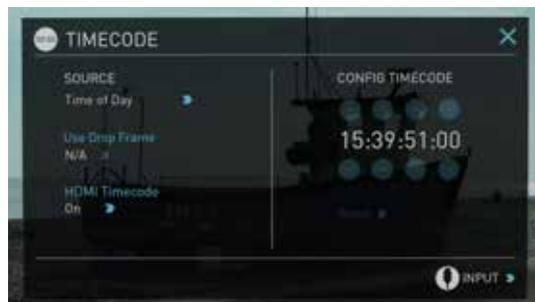
With this setting, each new clip that is created will contain embedded Timecode starting with the time of day when the recording is started. Please check that Ninja Flame clock has been set correctly.
