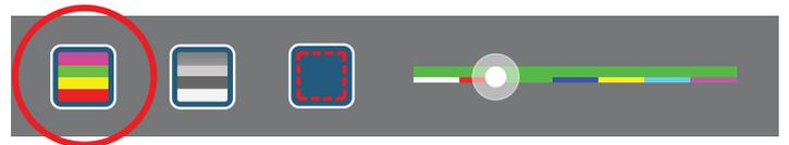
The Zebra threshold value can be adjusted by moving the slider left or right. The threshold percentage will be shown on the right of the slider.
