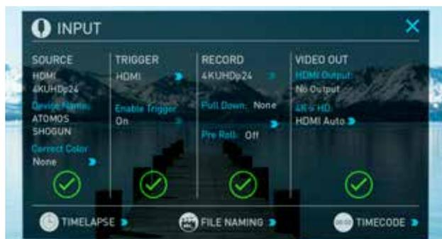
If the camera is Record Run mode, recording can be stopped or started by a moving Timecode via HDMI.
