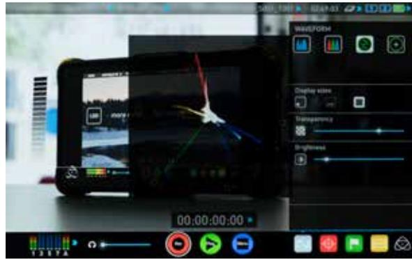
The Vectorscope display shows colour information of hue (shown as a phase vector), and saturation (measured by outward distance from the centre). This is useful for checking if an image is under or over saturated and for calibrating multiple cameras to ensure greater consistency between shots.
