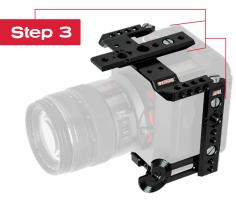
• Install the top by screwing in three 1/4"-20 screws, 1 into the top of the camera and 1 into the top of each side piece.
