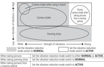
Set the vibration reduction mode switch to either NORMAL or ACTIVE.
