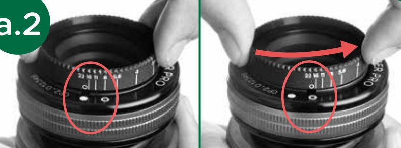
**EN** Align the hollow dot on the Optic with the solid dot on the lens body. Firmly grip with thumb positioned as shown, then push down and turn counter clockwise until the hollow dot on the Optic and the hollow dot on the lens body align.
