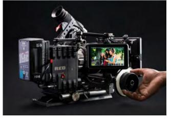
Construction note: Shinobi SDI is designed to operate in ambient temperatures up to 40°C/104°F. If you wish to extend the temperature of operation in high temperature conditions, set the TFT brightness to a minimum.
