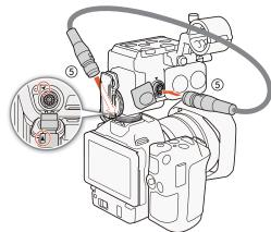
4 Put the unit cable through the cable clamp (6).
