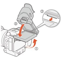
4 Hook the viewfinder unit latch under the left side of the LCD panel and then fasten the latch. Then, return the LCD panel to its original position.
