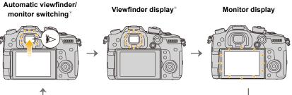
\* If [Eye Sensor AF] in the [Custom] ([Focus / Release Shutter]) menu is set to [ON], the camera automatically adjusts the focus as the eye sensor is activated. The camera does not beep when focus is achieved with [Eye Sensor AF].
