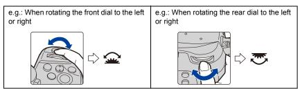
Allows you to set the aperture, shutter speed, and other settings when in  $\, {\bf P} \, / \, {\bf A} \, / \, {\bf S} \, / \, {\bf M} \,$  modes.
