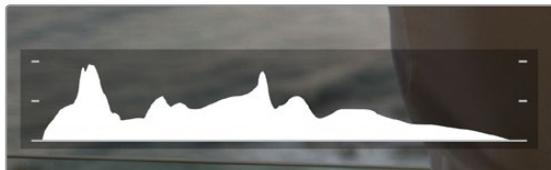
The histogram gives you an indication of the tonal range between shadows and highlights in your clip. It is also a helpful tool for checking the balance of your exposure and to prevent your highlights from clipping
