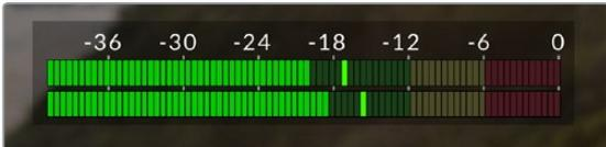
The colored bars on the audio meter represent peak audio levels. Ideally your peak audio levels should fall in the upper end of the green zone, between -20 and -12dBFS. If your peaks enter into the yellow or red zones, corresponding to -12 and -6dBFS your audio is in danger of clipping
