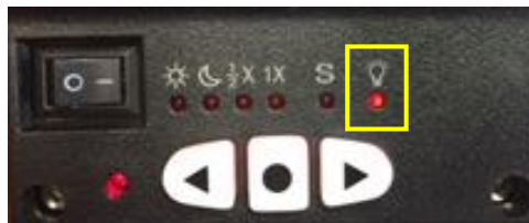
Figure 22 Polar scope LED intensity adjustment
