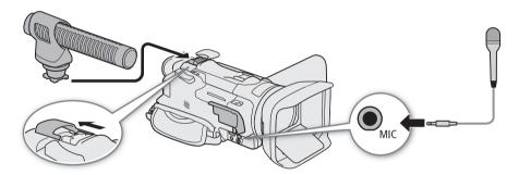
Attach the optional DM-100 Directional Stereo Microphone to the mini advanced shoe ( $\square$  70). Connect other external microphones to the MIC terminal.
