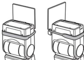
You can attach the plate to either side of the electronic flash.
