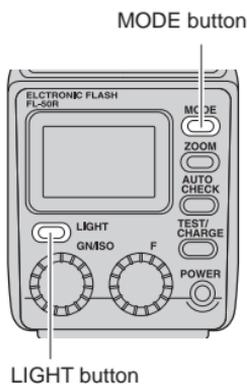
**1** Press the MODE and LIGHT buttons simultaneously for 2 or more seconds to reset to default settings.
