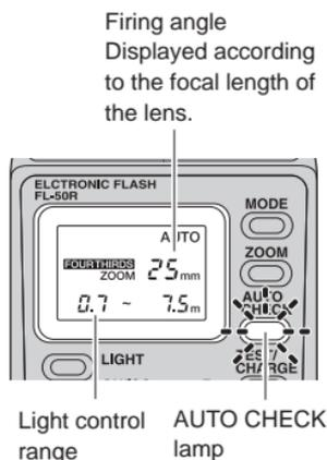
**1** The control panel shows the light control range according to the camera's setup.
