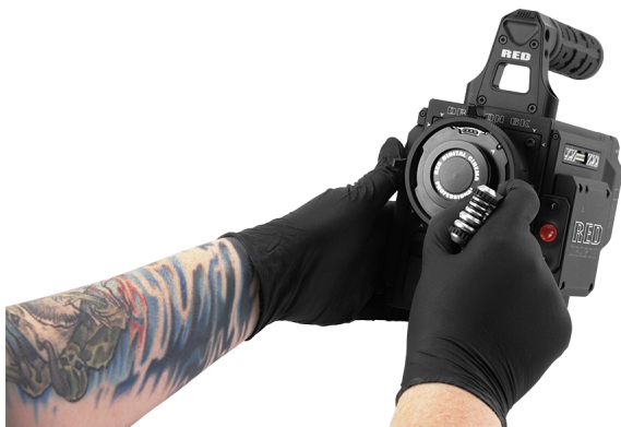
Figure: Remove the Lens Mount Screws
