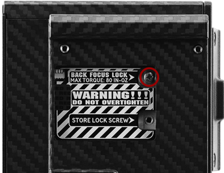
Figure: Back Focus Successfully Locked
