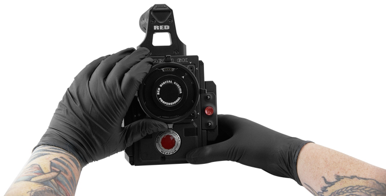
Figure: Turn Locking Ring Counter-Clockwise
