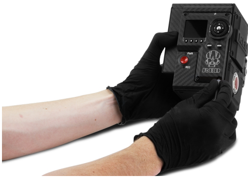
Figure: Remove the Side Module/Panel
