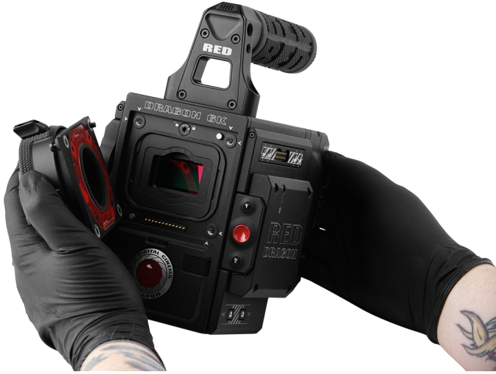
Figure: Remove the Lens Mount
