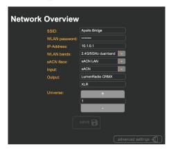
All configuration of the Apollo Wireless DMX Bridge can be performed using its integrated web based control panel. To access this:
