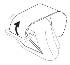
**5.** Wrap the strap tightly around the weight and attach to itself.
