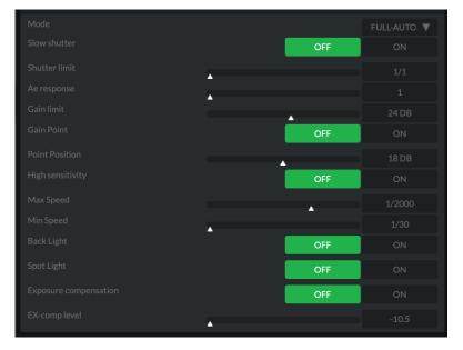
**Shutter Pri**: Shutter Priority mode. This mode allows you to set a fixed shutter SPEED with exposure achieved by automatic setting of IRIS and GAIN, according to the brightness of the subject. The exposure is adjusted automatically using the values manually set for SPEED, GAIN LIMIT, AE SPEED, BACK LIGHT, SPOT LIGHT and EXPOSURE COMPENSATION.
