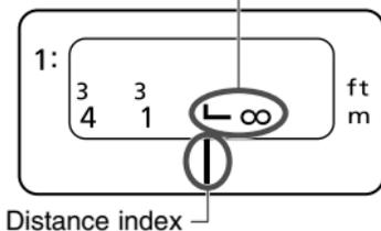
To compensate for shifting of the infinity focus point that results from changes in temperature. The infinity position at normal temperature is the point at which the vertical line of the L mark is aligned with the distance indicator on the distance scale.
