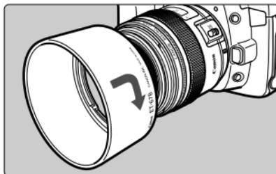
Attach and align the hood to the hood mount on the front of the lens, and turn the hood as shown by the arrow to secure it.
