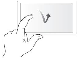
An operation to press and release the LCD monitor. An item or icon can be selected, or an item can be executed.
