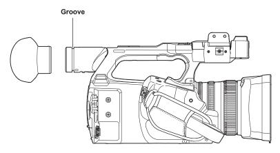
1 Attach the eye cup by aligning the groove on the attaching part of the eye cup with the inner ridge of the eye cup.
