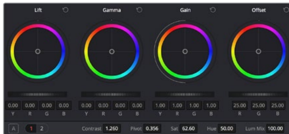
The 'lift', 'gamma', 'gain' and 'offset' and offset color wheels give you total control over the color and tonal balance of your clips. To make a uniform adjustment to all colors for each tonal region, drag the dial underneath the color wheels back and forth.
