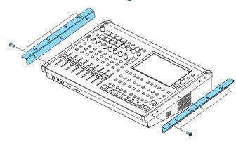
\* Both rack-mount angles are of the same shape, with no difference between left and right.
