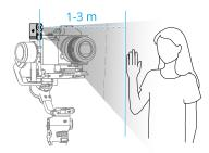
Adjusting composition: Adjust the composition as needed during tracking. Show the gesture to the camera. The indicator turns solid yellow and tracking is automatically paused. The subject can move to the desired position in the frame.
