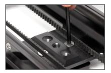
**Step 5**Loosen rail knobs and angle Parallax rail away from drag end of the slider
