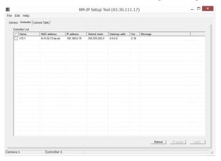
7. Select the [Camera Table] tab, then select the remote controller you want to set from the [Controller] pull-down menu.
