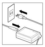
Connect the AC cable to the AC adapter.
