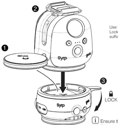
**i** Ensure the Genie Pan Tilt is locked in place once installed.
