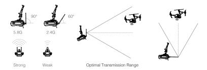
Ensure the aircraft is flying within the optimal transmission range. Adjust the distance and position between the operator and the aircraft to achieve optimal transmission performance. The position of the antennas required for optimal transmission range varies in the frequency of 5.8G and 2.4G. Please place the antennas based on the actual operating frequency.
