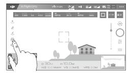
3. Tap once on the target direction and wait for icon to appear. Tap again to confirm the selection and the aircraft will automatically fly towards the target direction.
