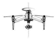
Hold the aircraft vertically, with nose pointing downward, and rotate it 360 degrees around the center axis. Recalibrate the compass if the Aircraft Status Indicator glows blinking red.
