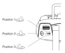
P-mode (Positioning): P-mode works best when the GPS signal is strong. The aircraft utilizes GPS, stereo Vision System and Infrared Sensing System to stabilize, avoid obstacles or track moving subjects. Advanced features such as TapFly and ActiveTrack are enabled in this mode.
