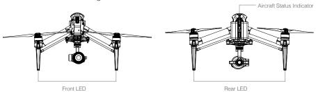
The Front LEDs show the orientation of the aircraft. The Front LEDs glow solid red when the aircraft is turned on to indicate the front (or nose) of the aircraft (Front and rear LEDs can be turned off in the DJI GO 4 app). The Aircraft Status Indicator communicates the system status of the flight controller. Refer to the table below for more information about the Aircraft Status Indicator.
