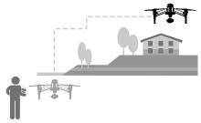
The aircraft automatically adjusts its speed when it senses an obstacle in front, or if it flies too close to the ground. The DJI GO 4 app will show a prompt if the aircraft flies over an obstacle or to the left or right of the obstacle. However, this feature should not be relied upon for navigation between obstacles. Failsafe procedures will override TapFly. If the GPS signal weakens, the aircraft will exit autonomous flight and return to home.
