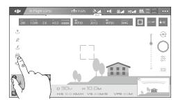
3. Tap on the subject you want to track then tap to confirm selection. If the subject is not automatically recognized, drag a box around it. The box is will turn green when tracking is in progress. If the box turns red, the object could not be identified and you should try again.
