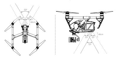
riangle The aircraft cannot detect objects in shadow. Fly carefully.
