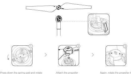
the propeller lock until the arrows are aligned and you hear a click.
