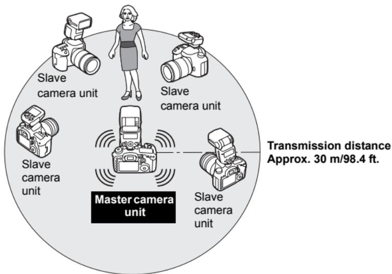
Before performing the operations on the next page, attach a Speedlite or transmitter to all the cameras to be used for linked shooting. For details on setting other devices, refer to the instruction manuals of the devices.
