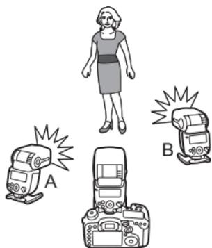
You can divide the slave units into two firing groups, A and B, and adjust the lighting balance (flash ratio) for shooting. The exposure is controlled automatically so that the total flash output of firing groups A and B results in the standard exposure.
