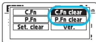
You can clear all Custom Functions or Personal Functions by selecting < **C.Fn clear** > or < **P.Fn clear** > on the screen on the left, and selecting < **OK** >.
