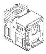
2 Insert an AXS memory card into the card slot with the label facing the direction shown in the diagram.
