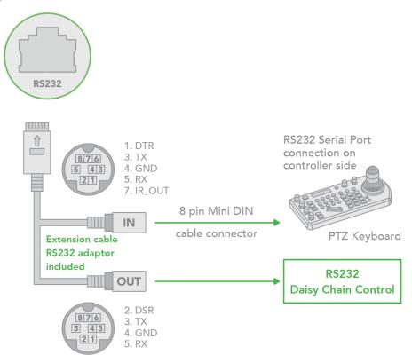
6. Use the included RJ45 to RS422/232 cable with a Phoenix terminal contact adaptor to make an RS232 connection for your control device.
