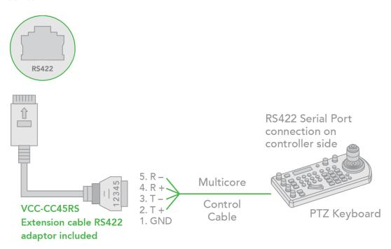
b. Use a CAT5/6 T-568B cable for an RS422 direct connection between the camera and the controller by following the pin definition below.
