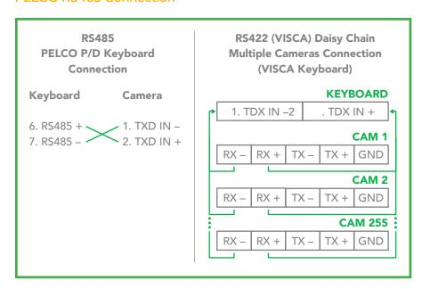
a. Use the included RJ45 to RS422 cable with a Phoenix adaptor to make an RS485 connection for your control device.
