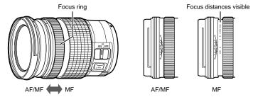
focus even when the MF clutch is in the MF position.
