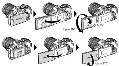
· Gently rotate the monitor within its range of motion. Attempting to rotate the monitor beyond the limits shown below could damage the connectors.
