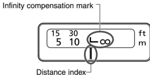
To compensate for shifting of the infinity focus point that results from changes in temperature. The infinity position at normal temperature is the point at which the vertical line of the L mark is aligned with the distance indicator on the distance scale.
