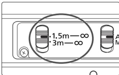
You can set the focusing distance range to 1.5 m/4.9 ft. to infinity or 3 m/9.8 ft. to infinity. By setting the suitable focusing distance range, the actual autofocus time can be shorter.
