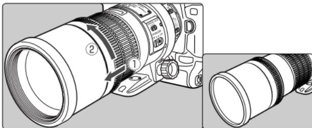
The built-in lens hood can reduce unwanted reflections and also protects the front of the lens from rain, snow, dust, and other substances. When using the hood, extend it outward from the end of the lens until it stops and then turn it in the direction of the arrow. For storage, reverse the procedure.
