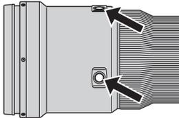
Set the focus-hold/prefocus switch to FOCUS HOLD and press the focus-hold button.
